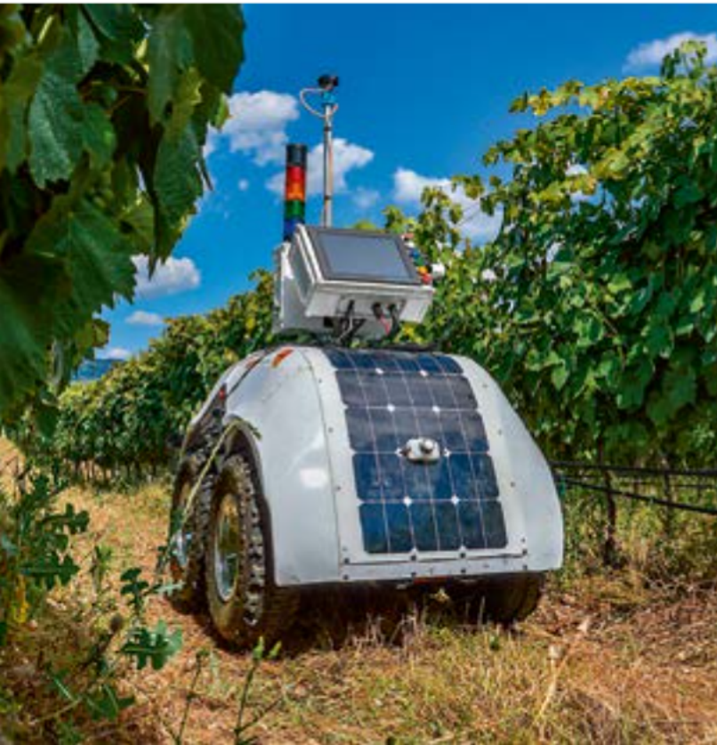
Computing and robotics open new possibilities for efficient crop management. The picture shows a robot developed by the Polytechnic University of Valencia (Spain) monitoring vineyard parameters like water availability, leaf temperature, and plant vigour.
