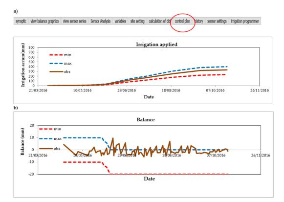
**Figure 4.** Screenshot of the 'control plan' tab of IRRIX in the year 2016, (**a**) the accumulated irrigation of treatment A during the irrigation campaign and (**b**) the water balance of treatment A during the irrigation campaign.
