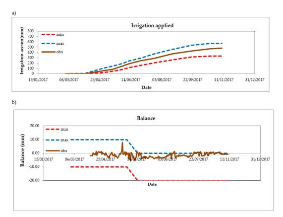
**Figure 5.** Screenshot of the 'control plan' tab of IRRIX in the year 2017, (**a**) the accumulated irrigation of treatment A during the irrigation campaign and (**b**) the water balance of treatment A during the irrigation campaign.
