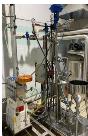
Figure 1. UHPH equipment used in this study for processing must and wine samples.
